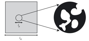
Figure 13. A typical porous medium illustrating the separation of length-scales, where  $l_p$  is the pore scale and  $l_m$  is the system scale.
