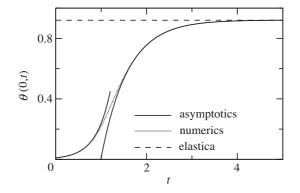
Figure 7.  $\theta(0,t)$  for P = 11,  $\delta = 1$ , Bi = 0.1, dx = 0.01, dt = 0.001 and  $\theta(x,0) = \theta(x,dt) = 0.01 \cos \pi x$ . The short-time asymptotic is for a growth rate s(P) found from equation (4.9). The long-time asymptotic is of the form  $Ae^{-\psi t} + \theta_0$ , where  $\psi$  is the rate of decay to the equilibrium angle  $\theta_0$  and A is a fitting parameter.
