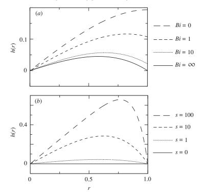
Figure 5. The radial variation of the fluid pressure at the onset of buckling, h(r), for (a) growth rate s = 1 and various values of the surface permeability parameter Bi (larger Bi corresponds to a more permeable surface) and (b)  $Bi = \infty$  and various s.
