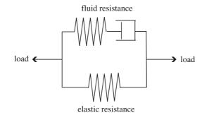
Figure 3. Mechanical analogue of the bending resistance of a poroelastic rod. For rapid displacements, the dashpot will not move and the fluid resistance due to the instantaneous pressure yields a response similar to a stiff (fluid) spring in parallel with an elastic spring. Eventually the dashpot will move to relieve the stress in the spring and the fluid resistance gradually decays, leading to a purely elastic steady state.
