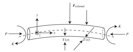
Figure 11. Schematic of a rod buckling under an applied twist and compression in an external medium. Y(x, t) and Z(x, t) are the displacements of the centreline in the y- and z-directions respectively. The dotted line denotes the axis of symmetry.
