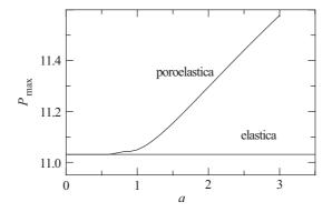
Figure 10. Maximum compressive load,  $P_{\text{max}}$ , for displacement-controlled buckling, where the displacement field is given by  $\Delta(t) \approx 0.1[1 + \tanh at]$ . Bi = 0.1,  $\delta = 1$ , dt = 0.01, dx = 0.01.
